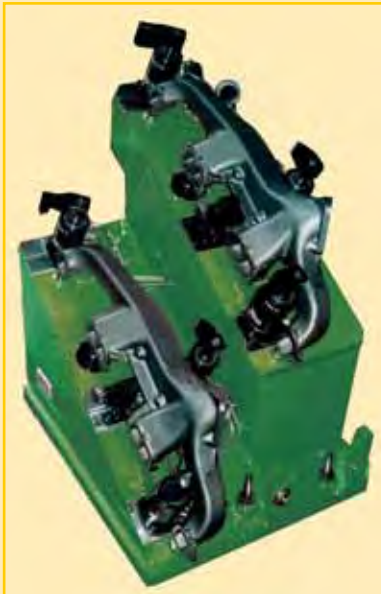
■ Fixture for machining exhaust manifolds.
