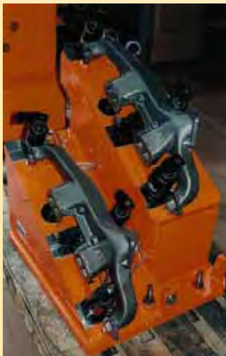
■ MPTL-100 and MPTR-100 Collet-Lok® Swing Clamps are used to securely clamp these exhaust manifolds.
